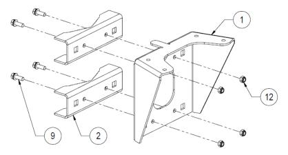
Assemble above sub-unit and item 8 to antenna by M8 washer and nut (with 11Nm / 8 ft-lbs torque). NOTE: The convex steeliness ring on item 8 MUST be inserted to end plate of antenna.
